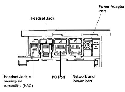
Figure 2: Ports on the Back of the 6910 IP Phone
